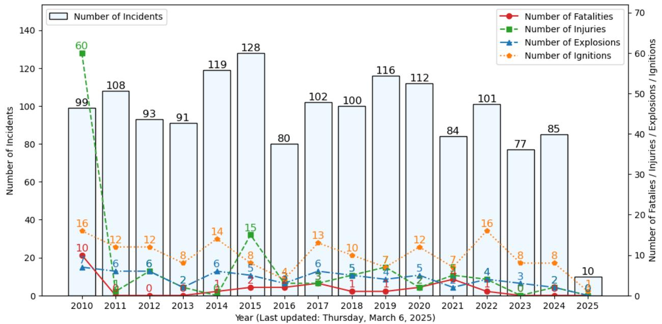
**Figure 2. Trends of Gas Transmission Incidents for Hydrogen and Natural Gas**
